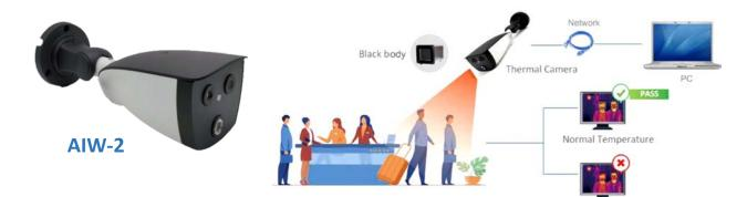
This Intelligent AI binocular thermal imaging system is composed of AI binocular temperature detecting camera and AI thermal imaging screening system.
