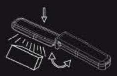
2 The sterilizer only works when the UV tube lamps are facing to the ground. It will pause the working automatically if the UV tube lamps are facing to the sky to avoid eyes damage.
